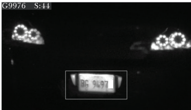
Washed Out and Over Exposed
